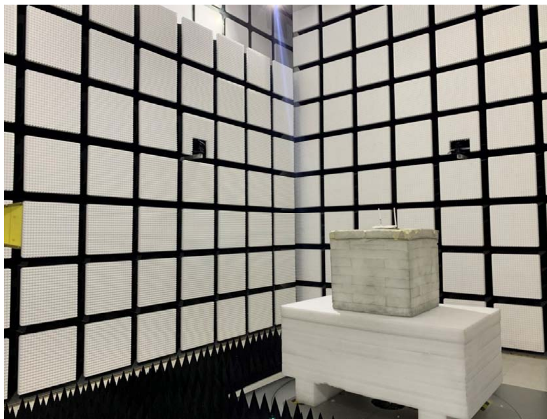
Radiated Emission Above 1GHz View
