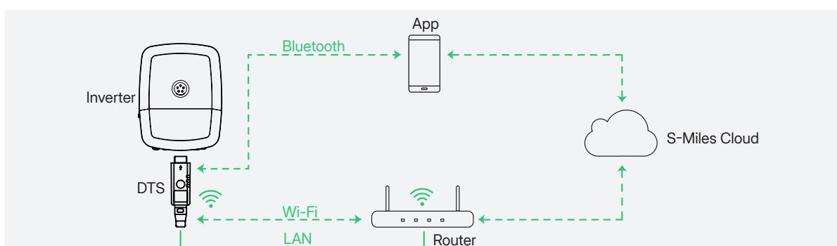
\* DTS Interface: Connect and communicate with the inverter.
