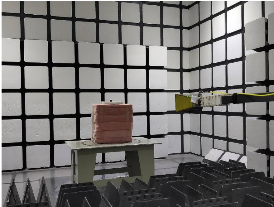
Radiated Emissions View (Above 1 GHz)
