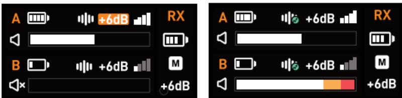
The A/B section on the home screen displays the status of transmitter 1 (TX1) / transmitter 2 (TX2).
