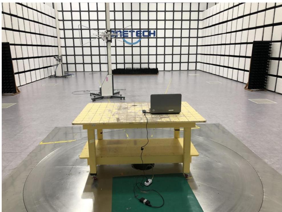
**- Radiated Emission Test (Above 1GHz)**
