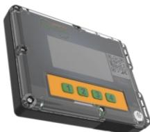
The SENTRY FlightSafe® is a reusable shipment tracking and monitoring device, allowing users to easily track location and sensor status.
