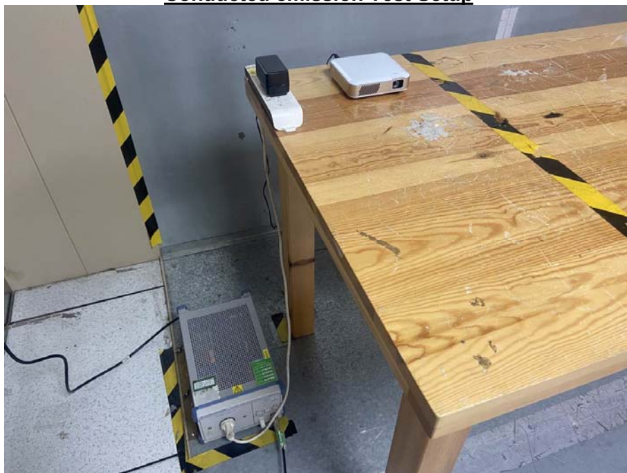
Conducted emission Test Setup
