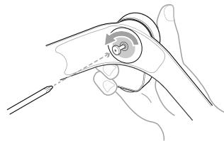
**Step 3:** Replace the DMAS Earphones and remount the screws.
