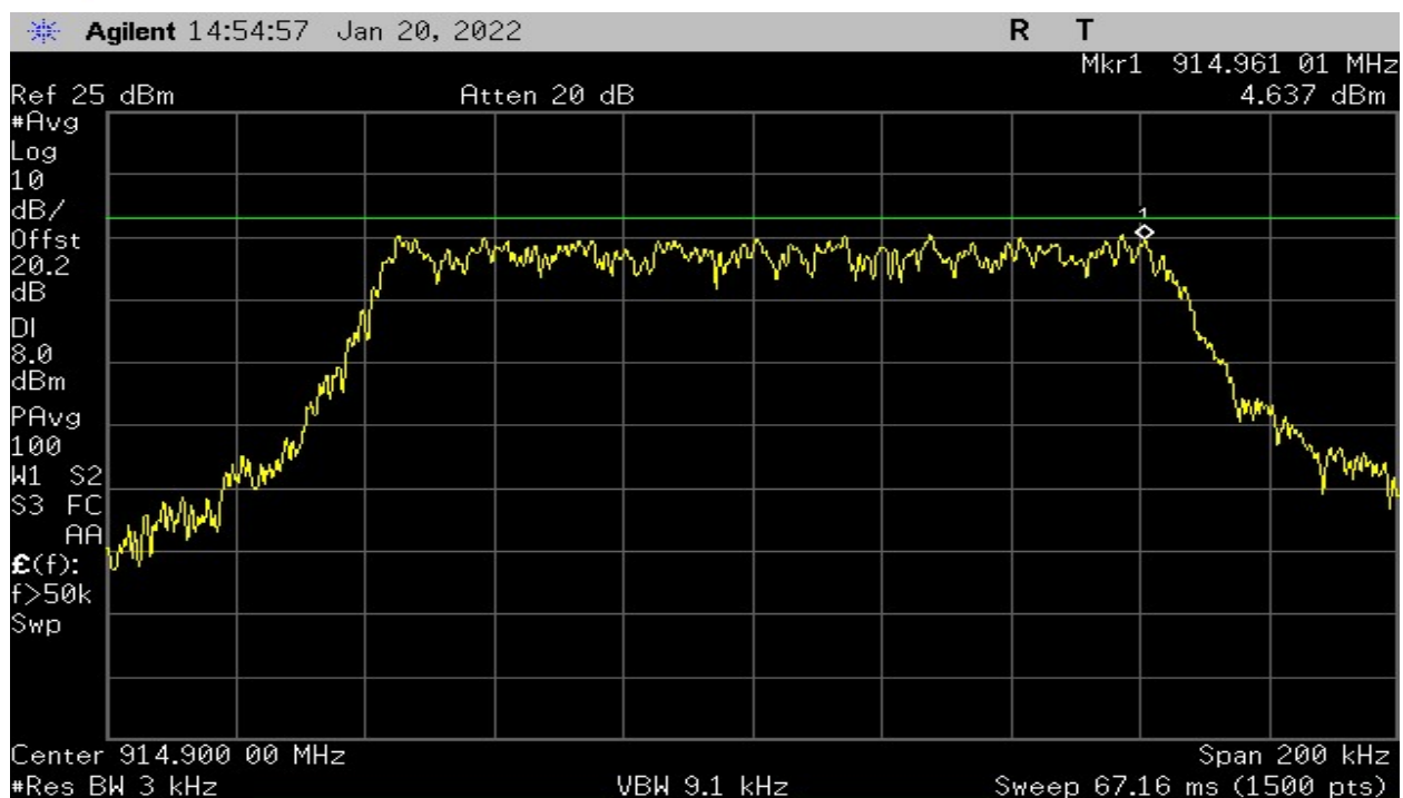
Plot 35 – Power Spectral Density – Highest Channel – 125kHz BW
