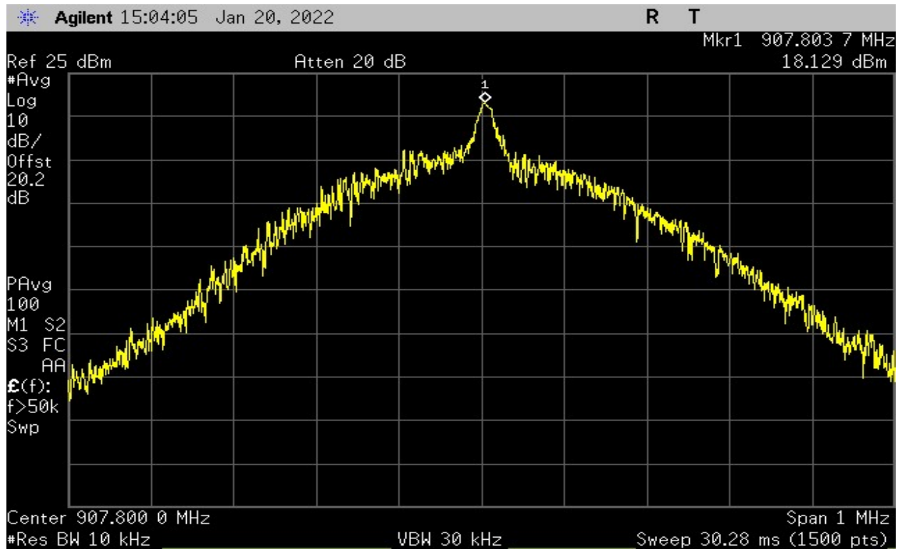
Plot 14 – Output Power – Middle Channel (500kHz BW)
