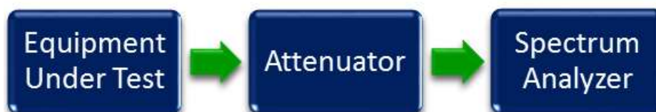
Figure 3. RF Power Test Setup
