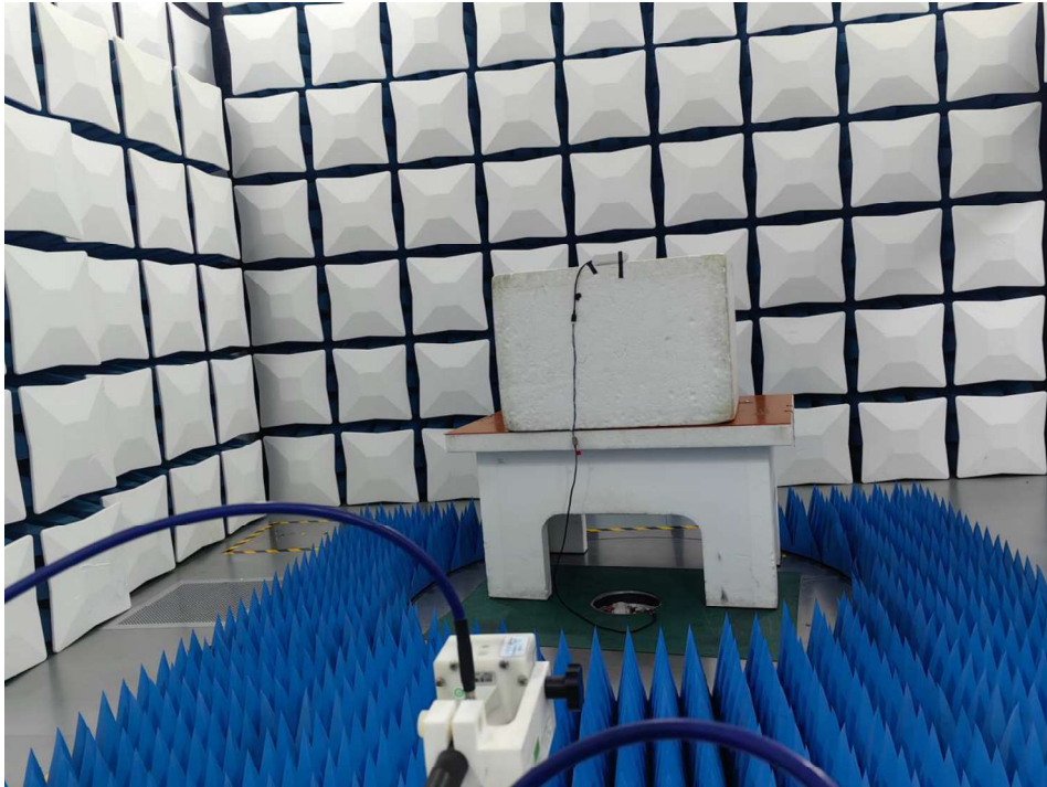
Test Set-up: Radiated spurious emission 18GHz to 40GHz
