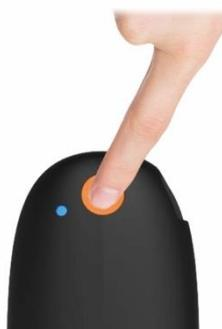
To switch BionicGym **ON** press the orange button for a second (the blue LED light goes on. The blue light flashes when it is trying to pair with the app and remains on when it is paired with the app).
