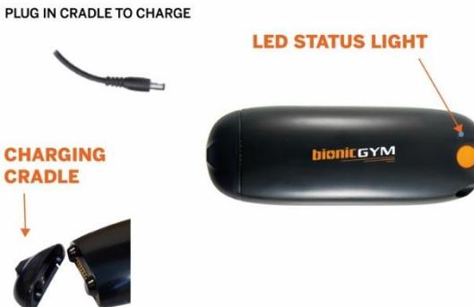
Assemble the charger (the adaptor twists into position) then plug **firmly** into the cradle. The cradle connects to the bottom of the control unit to charge. The battery takes an hour to 80% charged, and about two hours to charge fully.
