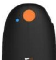
The session may also be paused by pressing the **orange button** on the control unit. Keep it pressed for 2 seconds to switch the unit off. Double press to resume the workout. The circle changes from white to orange as you progress through the session. If the unit loses connection with the App it may pause after a while (for safety reasons) and you may need to un-pause/restart the program. Even when the connection is lost, you can always stop a workout by pressing the orange button.
