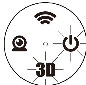
Long press the **Power** button, the power blue light will lighten the lights in the way of anticlockwise, until the light of **3D** and **Power** be lightened.
