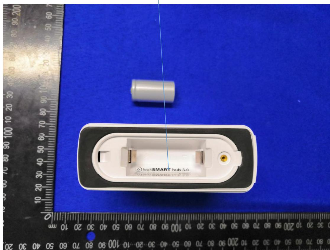
Note: label will be put on battery compartment and product will sold without battery installed. Label location also added in user manual page 11
