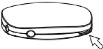
2. Replace the battery with a new one, make sure the positive terminal is facing up
