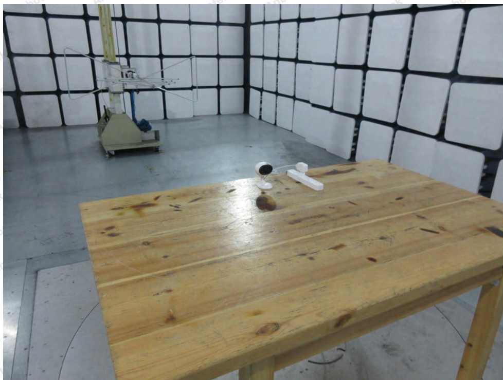
Photo of Radiation Emission Test
