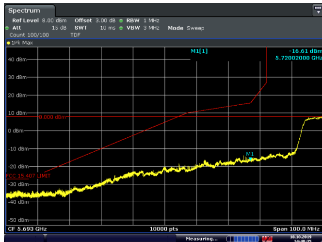
Figure 8.4-23: Band Edge measurement 5725 MHz VHT80 @ 5775MHz
