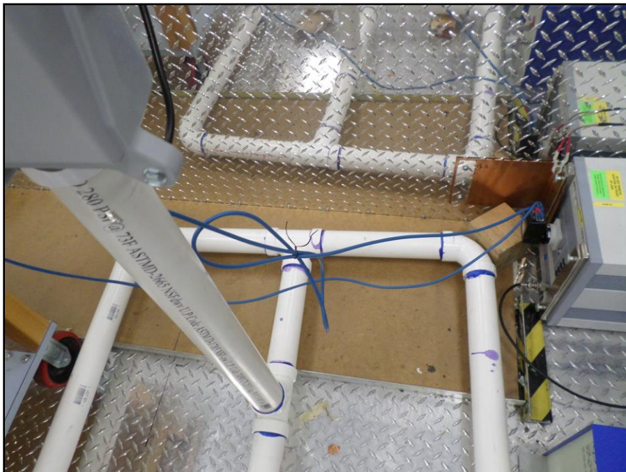
Photograph 2. Conducted Emissions, LISN Connection, Test Setup
