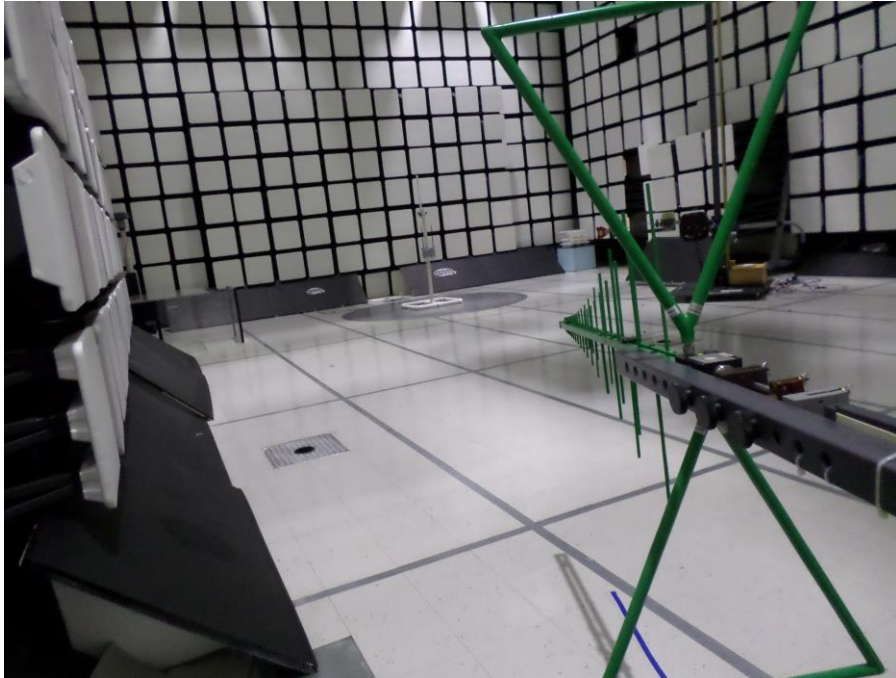
Photograph 4. Radiated Emissions, Setup Below 1GHz, Antenna
