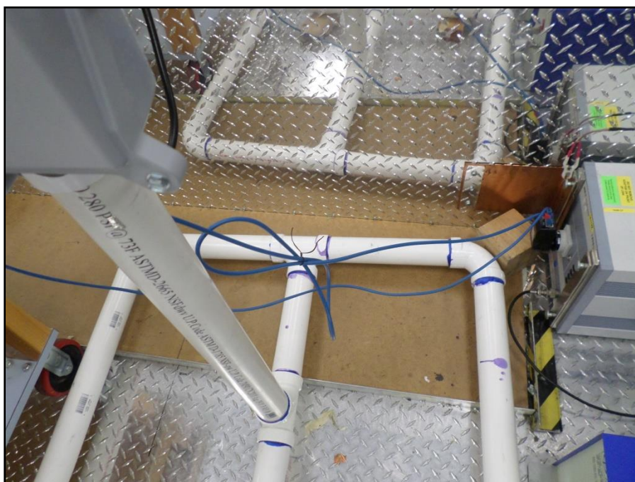
Photograph 2. Conducted Emissions, LISN Connection, Test Setup
