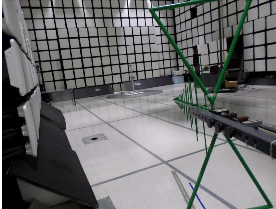
Photograph 4. Radiated Emissions, Setup Below 1GHz, Antenna
