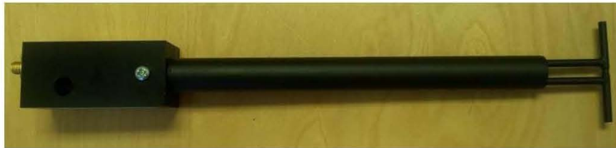
Figure 1 – MVG COMOSAR Validation Dipole
