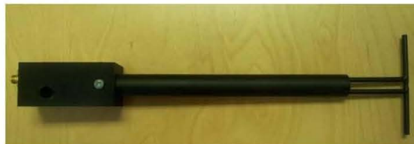
Figure 1 – MVG COMOSAR Validation Dipole
