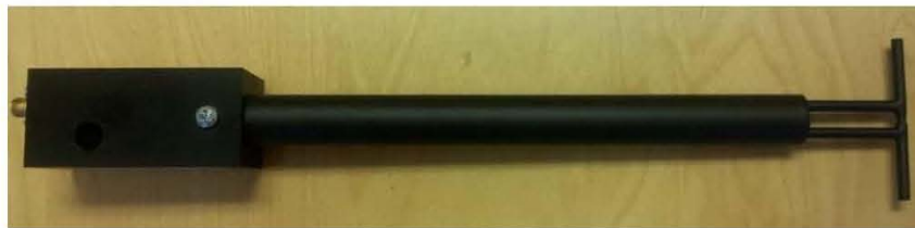
Figure 1 – MVG COMOSAR Validation Dipole
