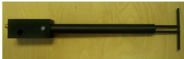
Figure 1 – MVG COMOSAR Validation Dipole
