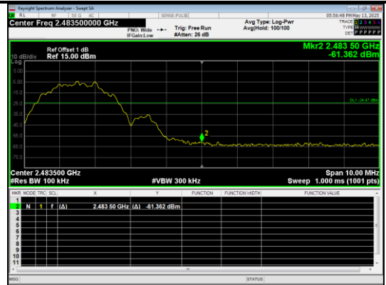
Out Of Band Emission BLE 2M_Channel 39
