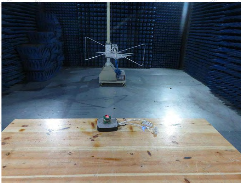
Photo of Radiation Emission Test
