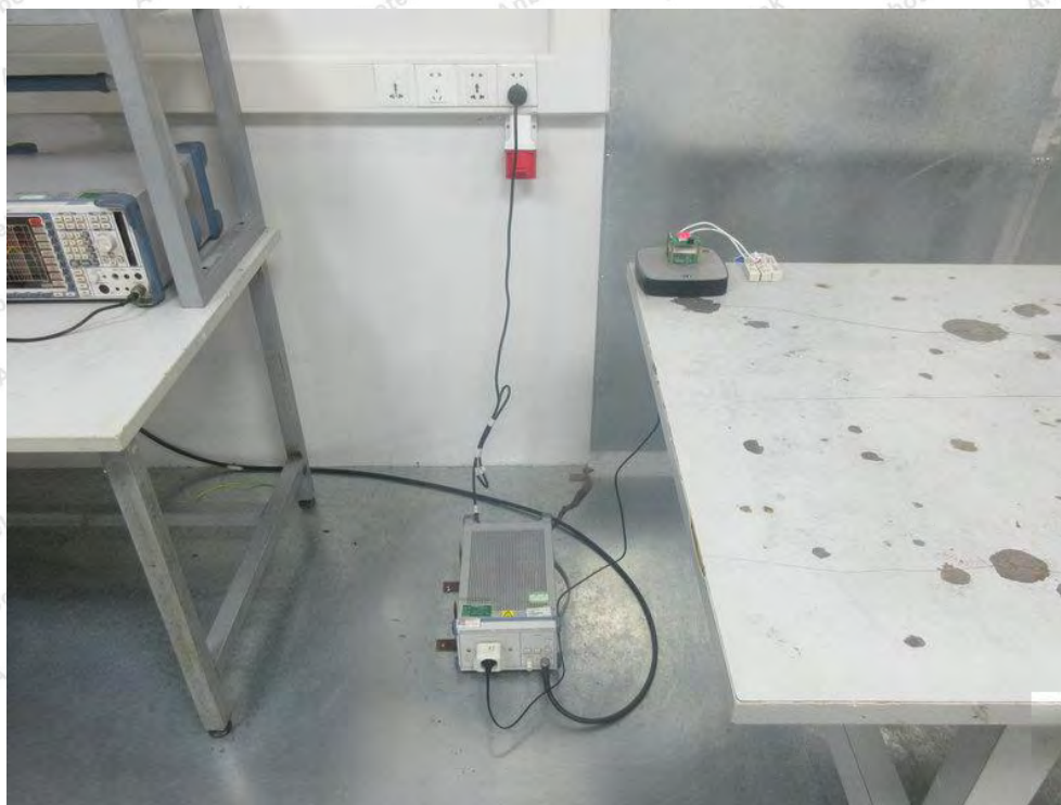
Photo of Conducted Emission Measurement
