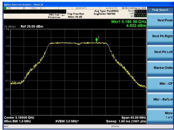
(802.11ac20) PSD plot on channel 40
