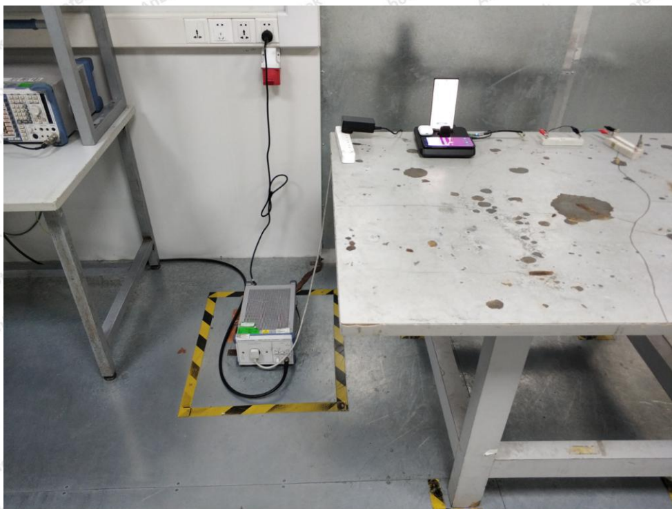
Photo of Conducted Emission Measurement
