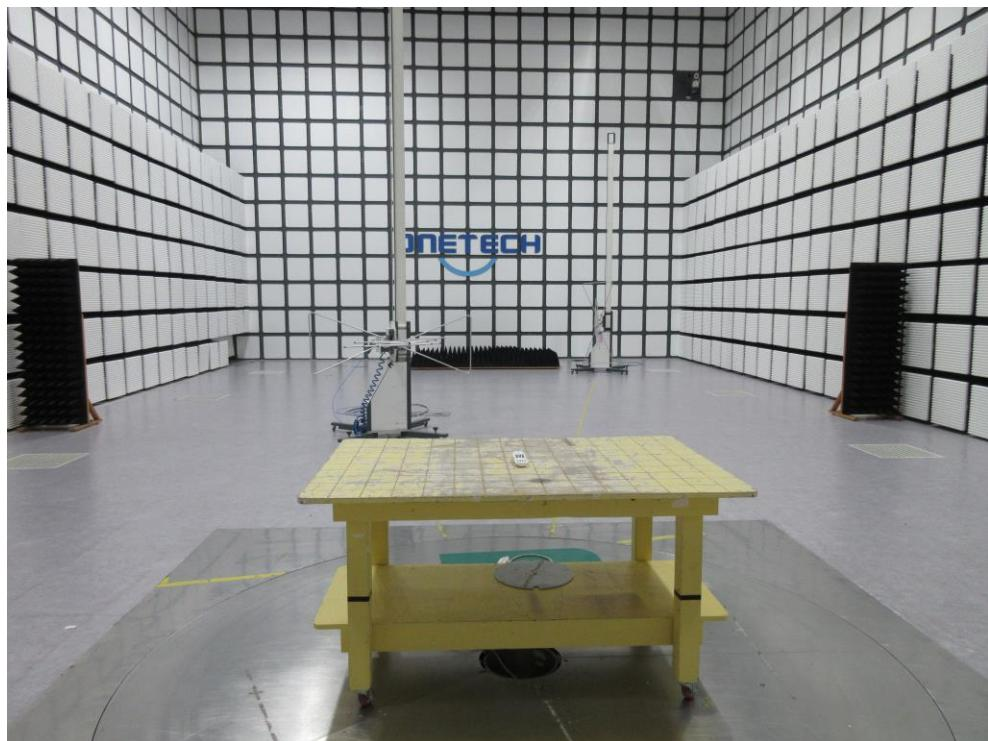
**- Radiated Emission Test (Above 1 GHz)**
