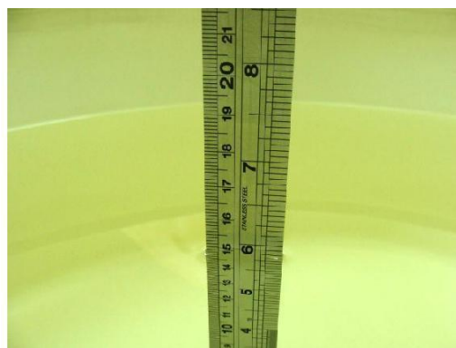
Fig 5.12 Photo of Liquid Height for Body SAR
