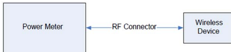
Figure 8.1.1 Power Measurement Setup
