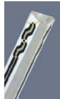
Figure 3.3 Probe Thick-Film Technique
