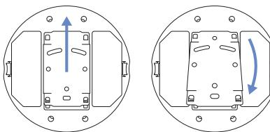
Push the Sensor towards the bracket and slide it until it is locked in place.
