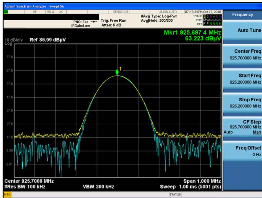
Note: The resolution bandwidth was set enough larger than occupied bandwidth of fundamental.
