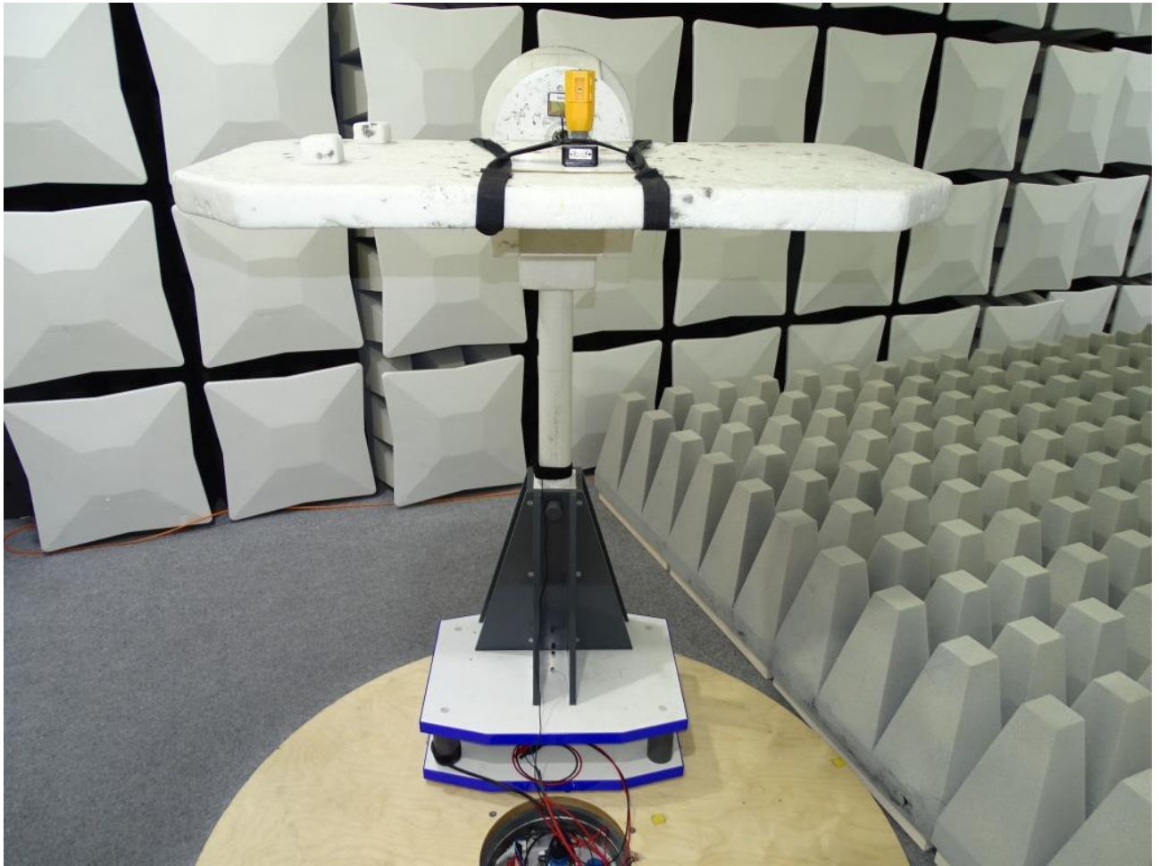
Photo 4: Test setup for radiated measurements above 1 GHz, right side view
