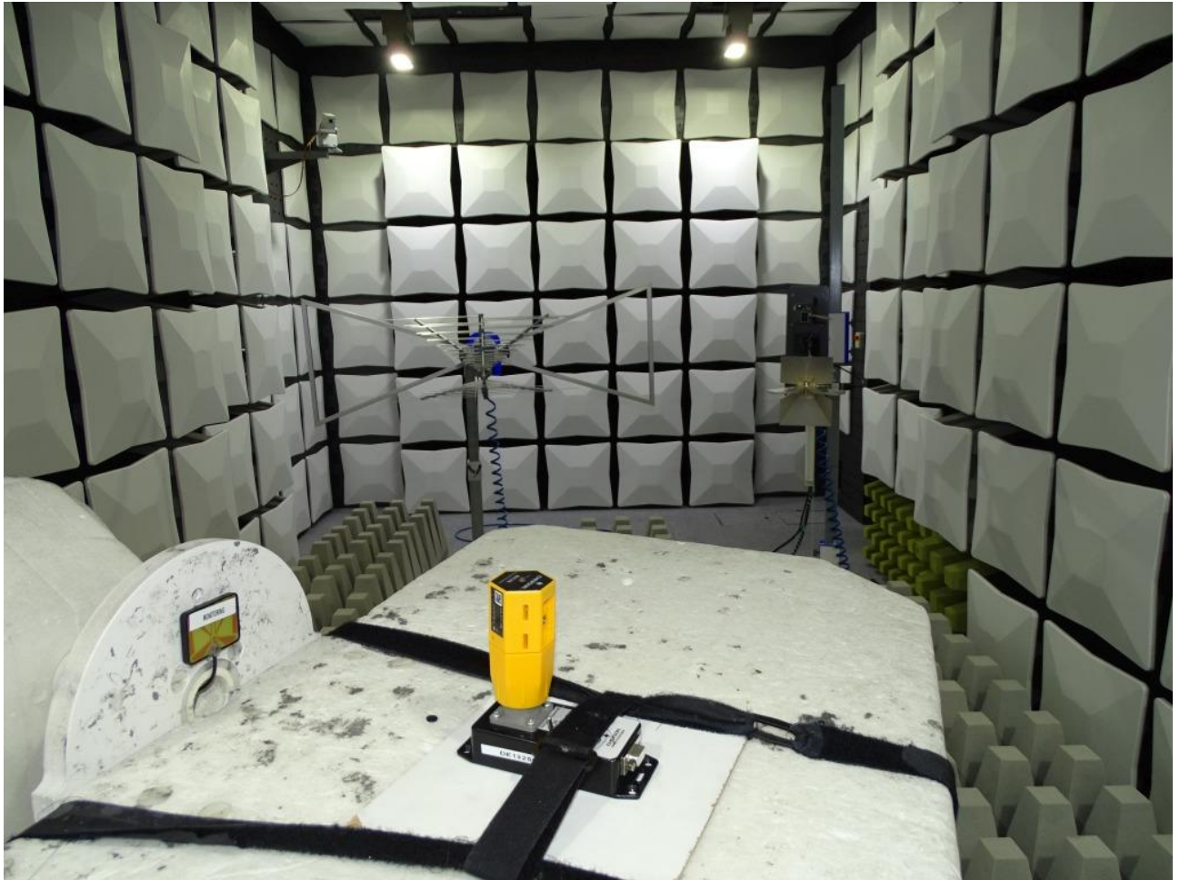
Photo 6: Test setup for radiated measurements above 1 GHz, detailed view
