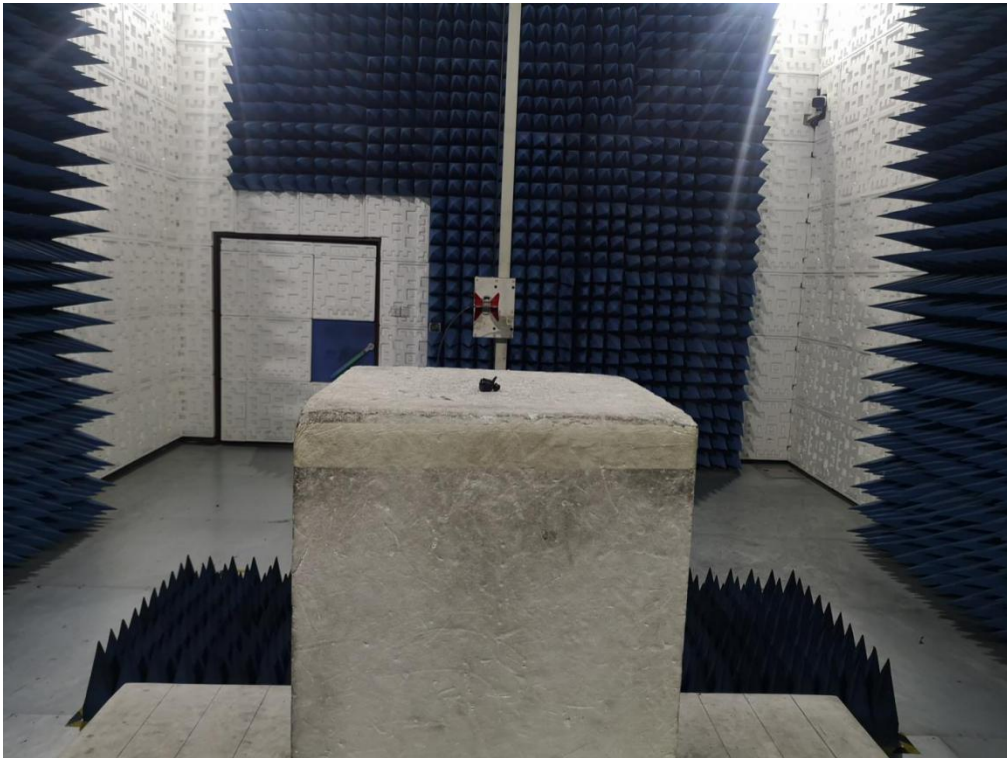
RADIATED EMISSION TEST SETUP ABOVE 1GHZ
