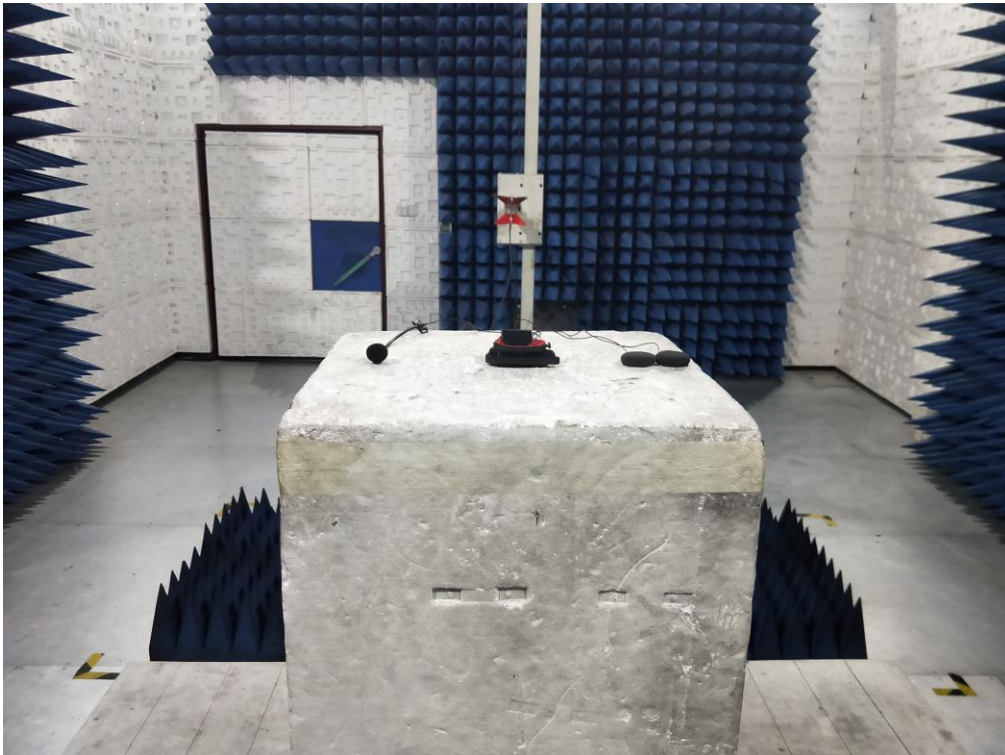
RADIATED EMISSION TEST SETUP ABOVE 1GHZ
