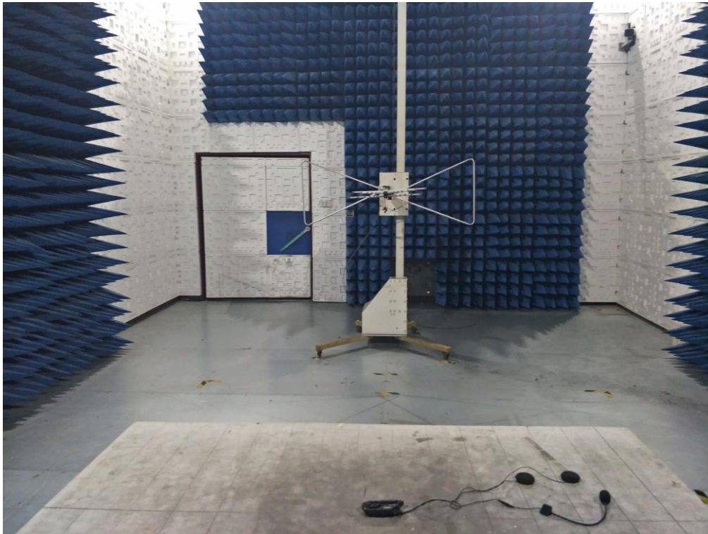
RADIATED EMISSION TEST SETUP ABOVE 1GHZ
