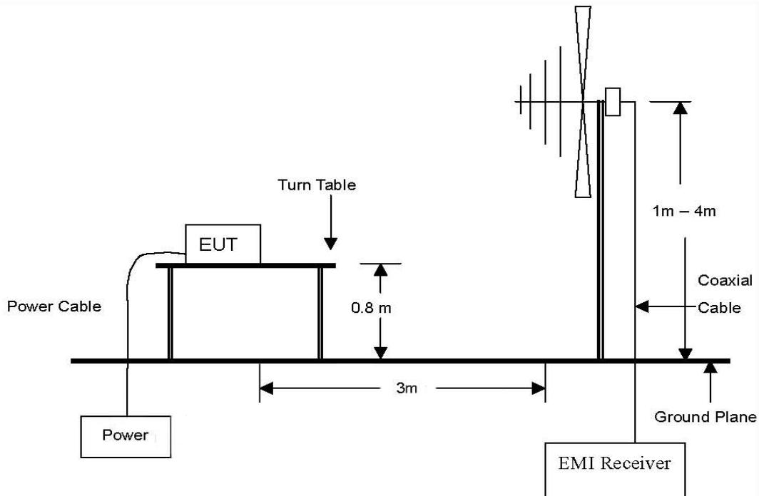
The diagram below shows the test setup that is utilized to make the measurements for emission from 1 GHz to 40 GHz emissions.
