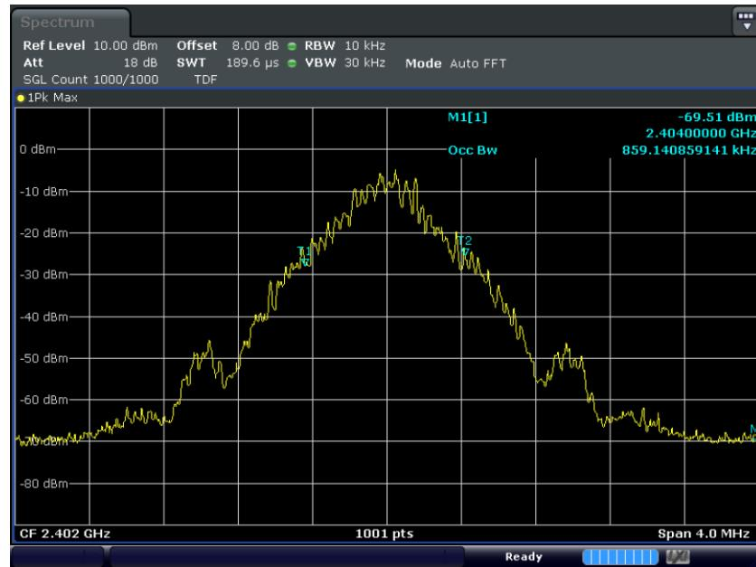
**B.1. Middle Ch. (2.441 MHz)\_20 dB Bandwidth**
