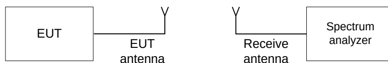
Figure 7.3.1 Occupied bandwidth test setup
