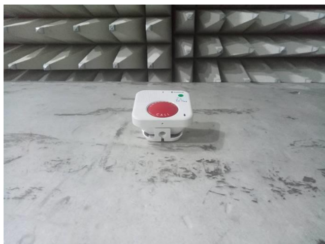
Photograph 8.1.2 Setup for radiated emission measurements, EUT cabling
