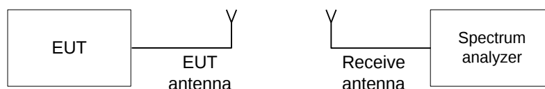
Figure 7.3.1 Occupied bandwidth test setup
