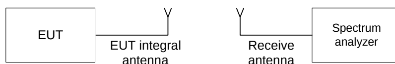
Figure 7.1.1 Setup for transmitter shut down test
