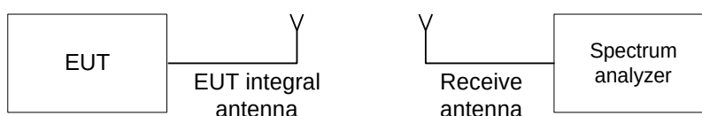
Figure 7.1.1 Setup for transmitter shut down test
