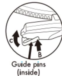
**STEP 1:** Hold the stylus at front edge(needle side) and insert the rear edge onto the tone arm(B).
