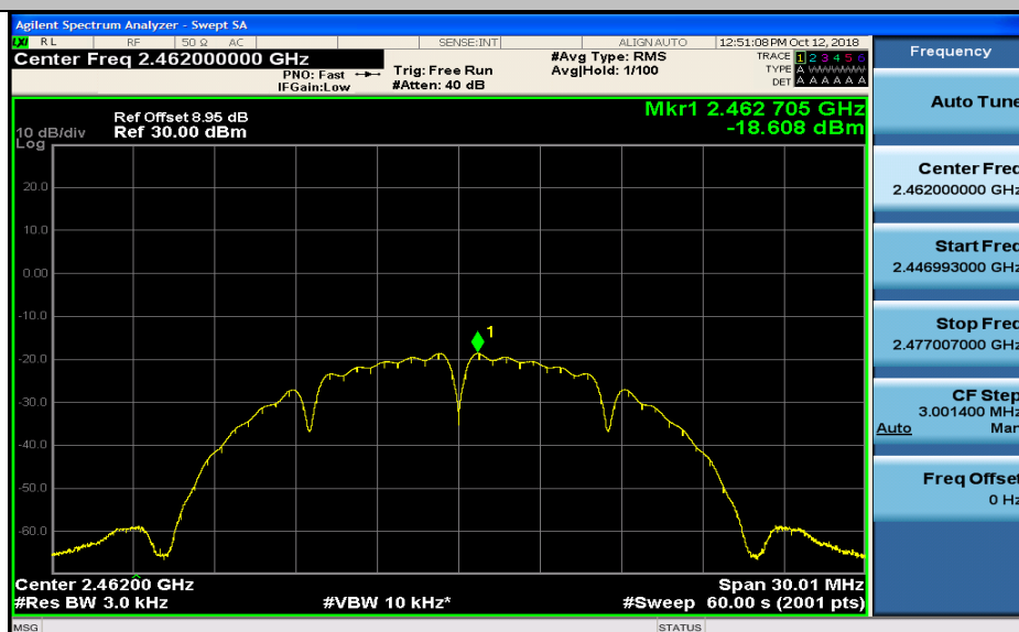
Maximum(average) power spectral density_11B_2462_Ant1
