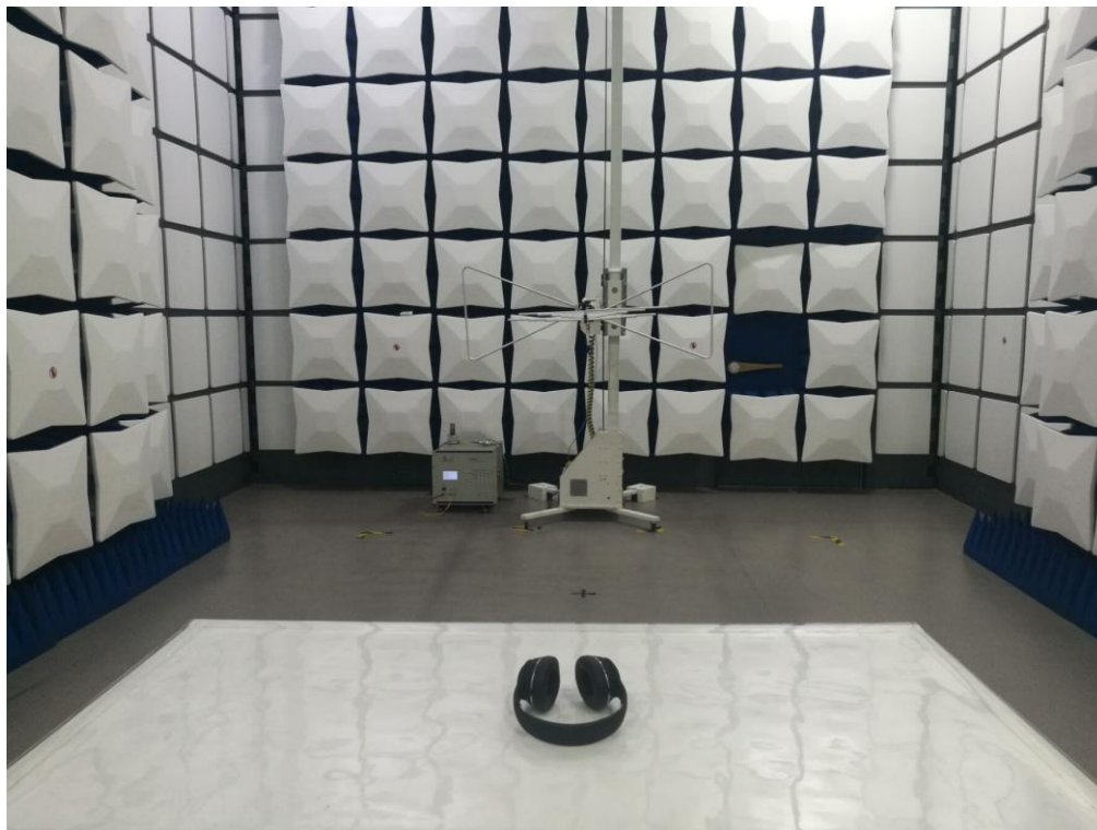
FCC RADIATED EMISSION TEST SETUP
