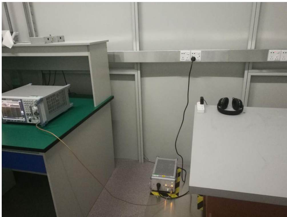
FCC RADIATED EMISSION TEST SETUP
