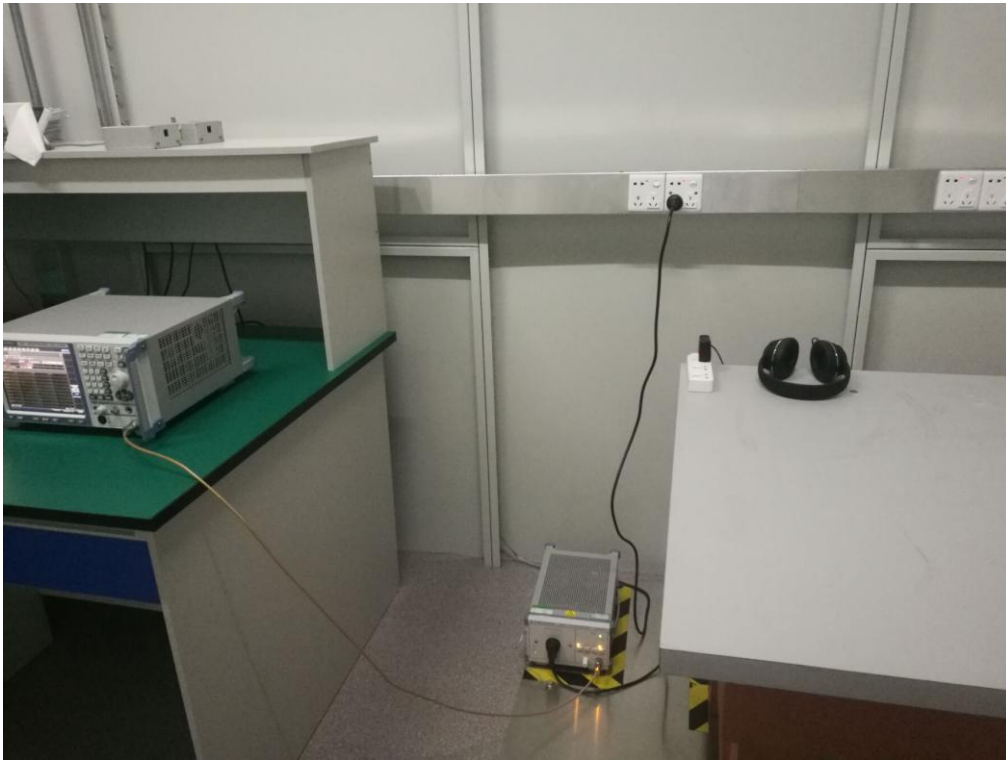
FCC RADIATED EMISSION TEST SETUP
