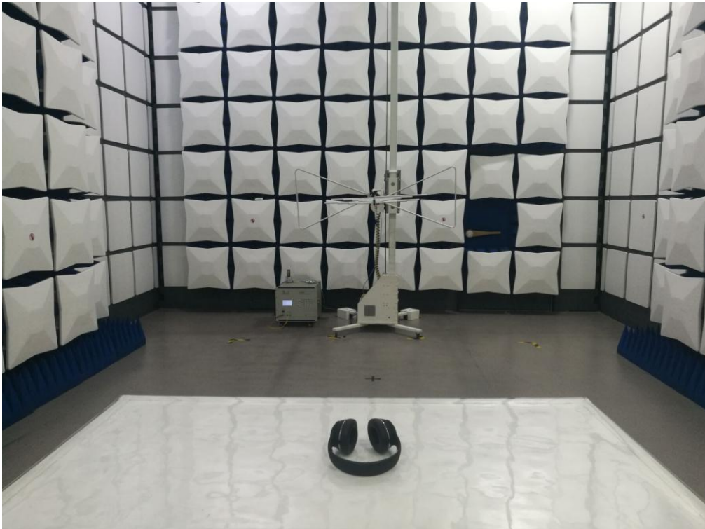
FCC RADIATED EMISSION TEST SETUP
