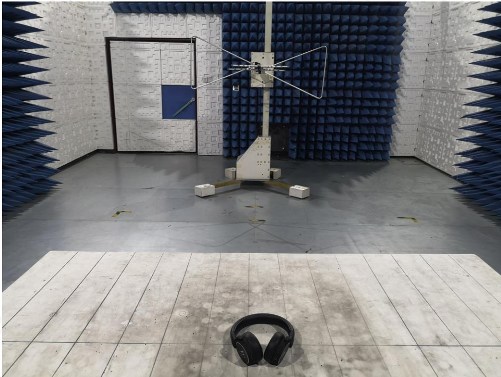
RADIATED EMISSION TEST SETUP ABOVE 1GHZ
