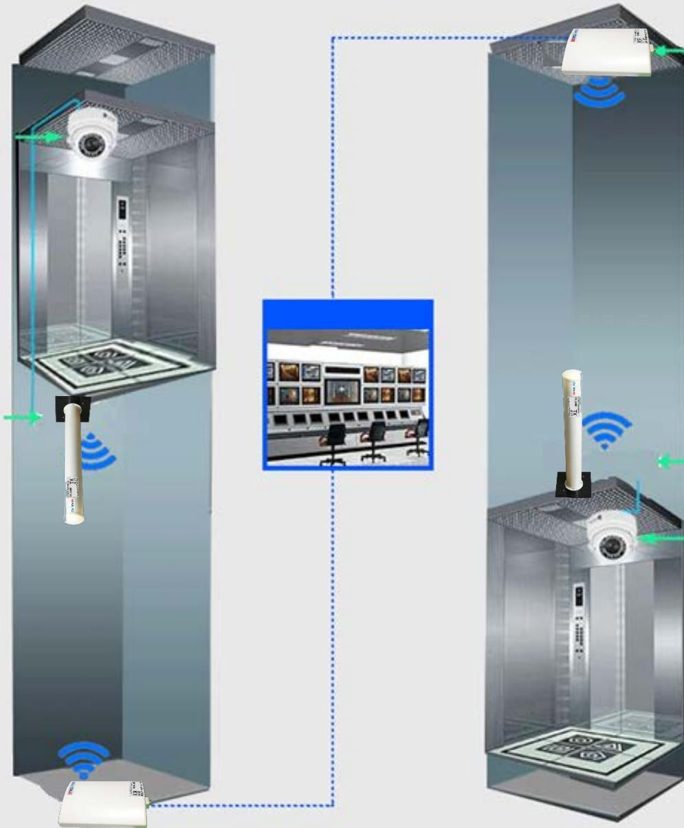
The antenna installation position is according to the control center. The RX box should install near the control center. The Transmitter and Receiver box are the same units. The manufacturer will setup in TX or RX mode and it would label it. So the installer will know the installation process.
