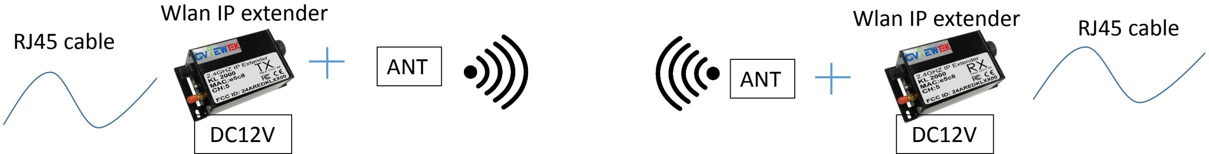
Turn on electricity after Wlan IP extender connecting with antenna. Should be aligned the transmitting antenna with the receiving antenna and not deviate from each other.
