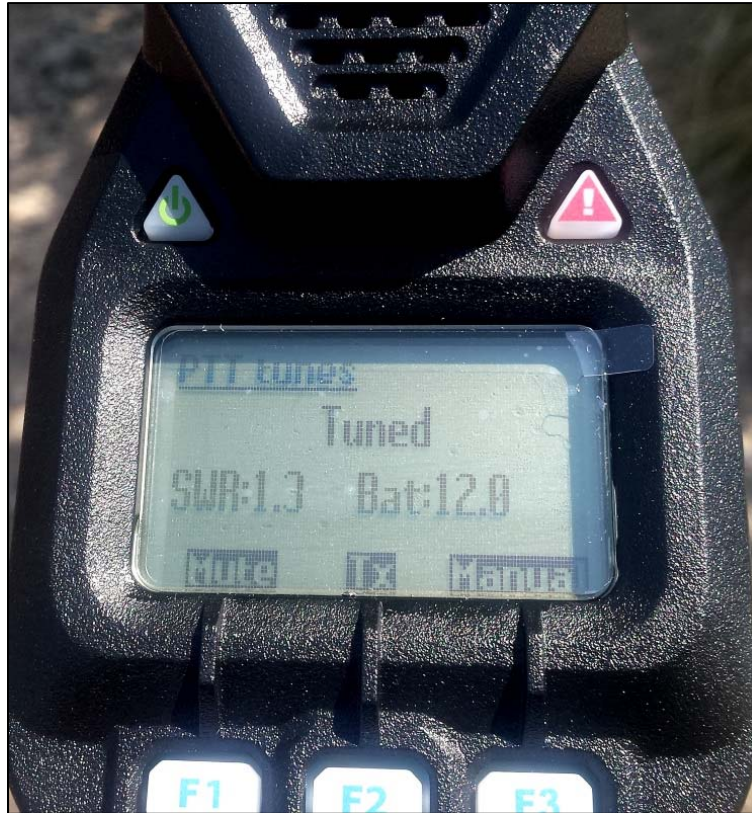
Figure 12. Antenna Status showing Tuned with a good SWR.
