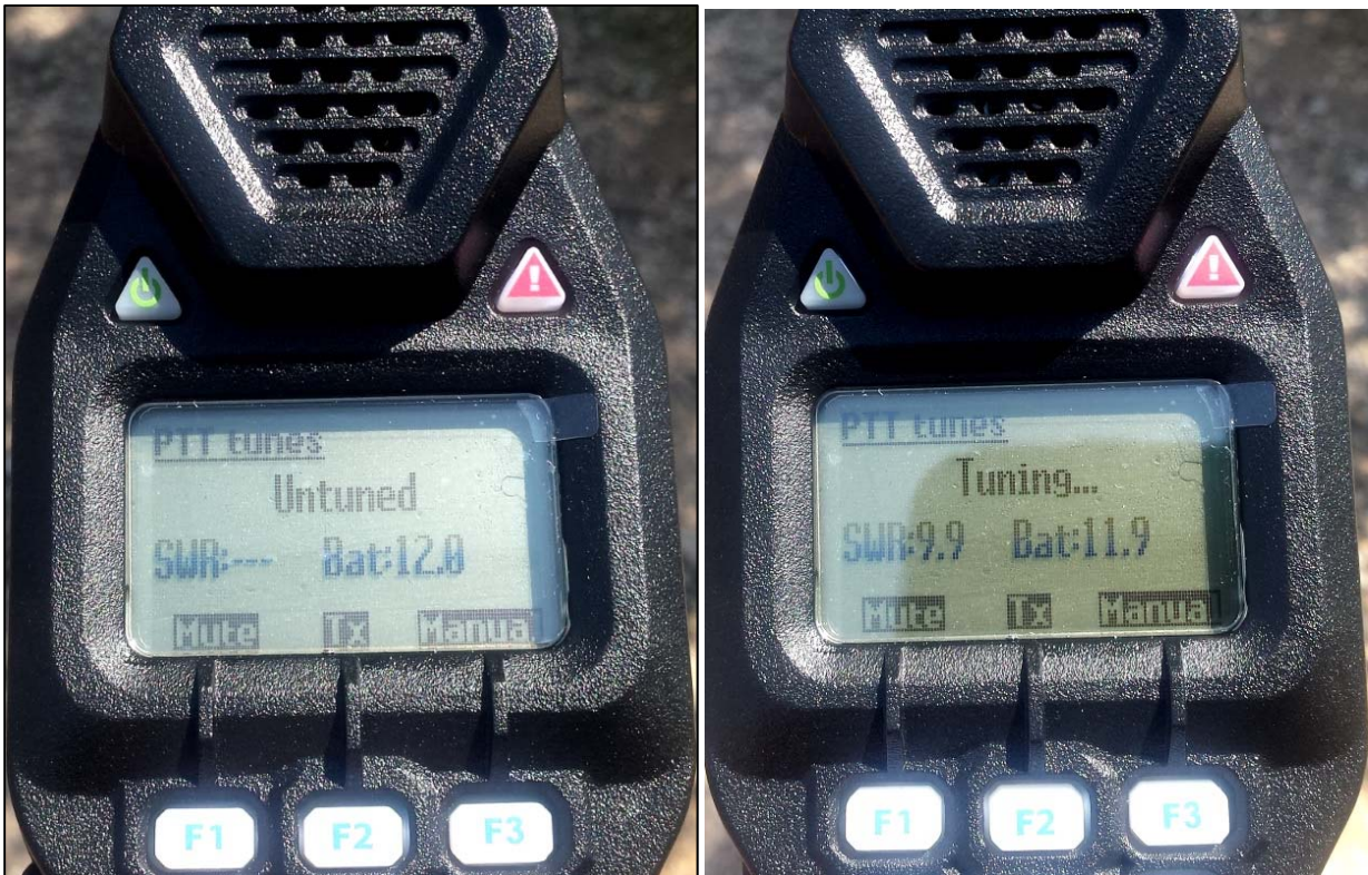
Figure 11. Antenna Status – Un-tuned and during Tuning.
