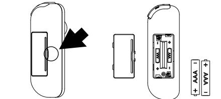
As Figure, open the back cover of the remote controller and install two AAA batteries (not included)
