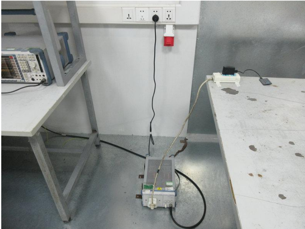
Photo of Power Line Conducted Emission Test
