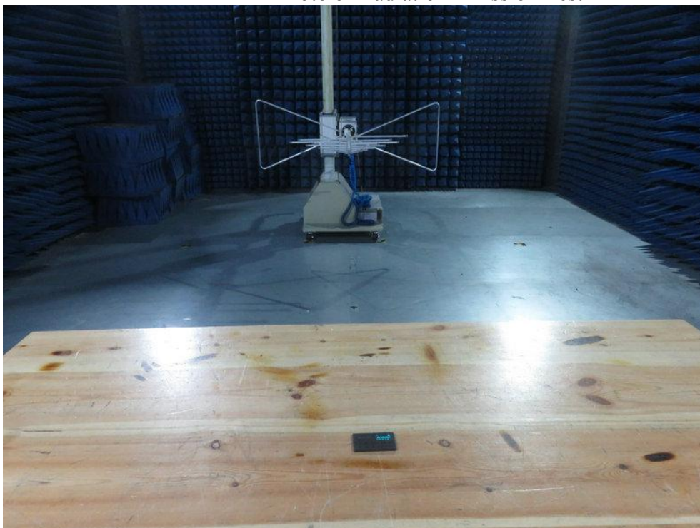
Photo of Radiation Emission Test
