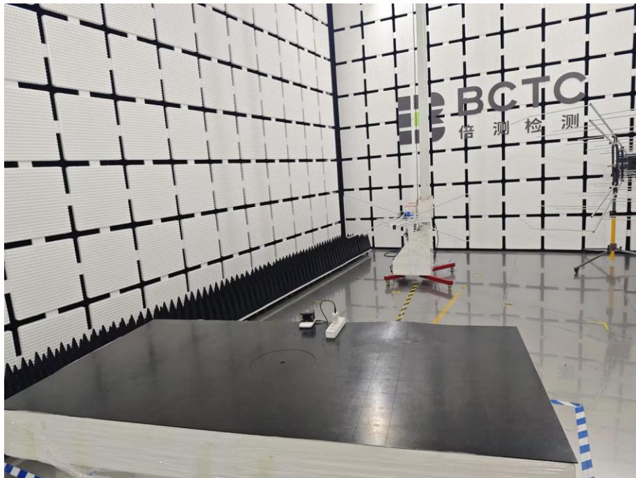
Radiated Measurement Photos 30MHz-1GHz
