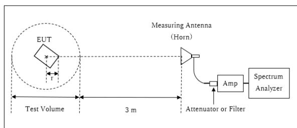
Distance Factor:  $20 \times \log (3.75 \text{ m}^* / 3.0 \text{ m}) = 1.9 \text{ dB}$
