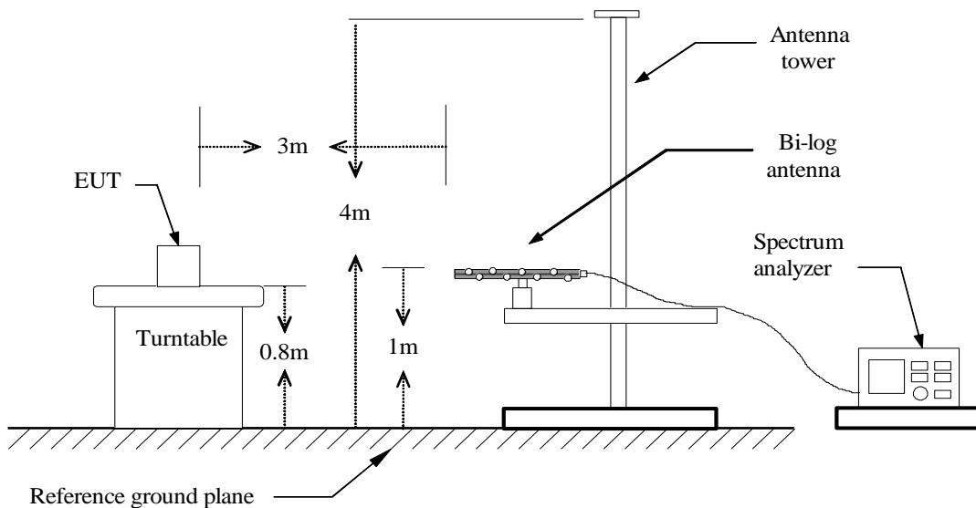
**Above 1 GHz**
