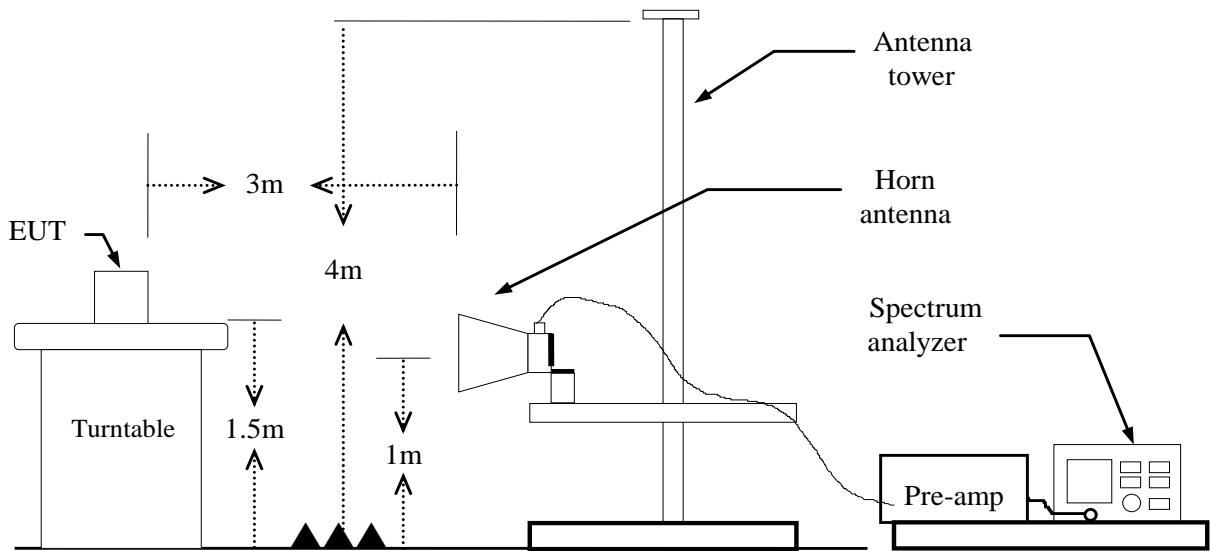
**Substituted Method Test Set-up**
